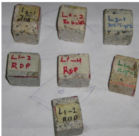
Fig. 1. The Rocks samples Cut to a regular dimension and set for the compression tests.
