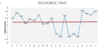
Fig. 9: System Response Time Plot for 20 different commands
