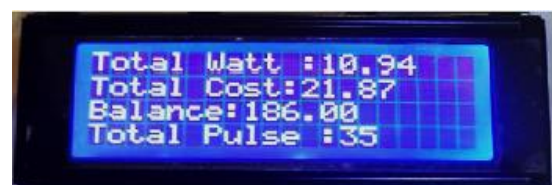
Fig. 10. Shows the total watt, cost, balance, and total pulse for 100 W load
