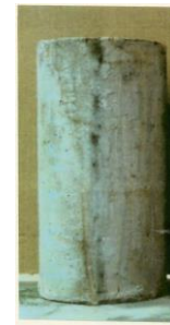
Fig. 3. Repaired Longitudinal Gap between New and Old Concrete.
