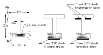
Fig. 1. Prestressed girder sections including CFRP.
