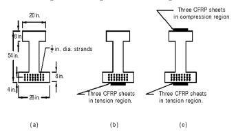
Fig. 2. Prestressed I-beam sections including CFRP.
