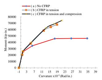
Fig. 5. Moment-curvature relations for the I-beam.
