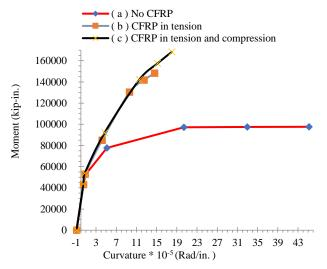
Fig. 4. Moment-curvature relations for the girder.
