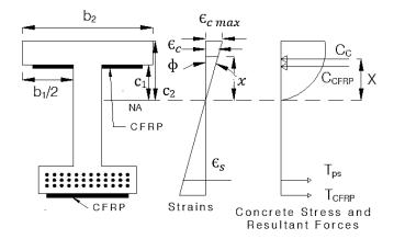
Fig. 3. Cross-Sectional strains, stresses and forces.
