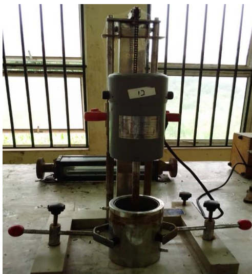
Fig. 3. The propellant mixer (Model: SWFS-400, Power: 400 watts, Voltage: 220 volts/50Hz, Size: 550×390×760 and Rotation speed: 0–8000 rpm).
