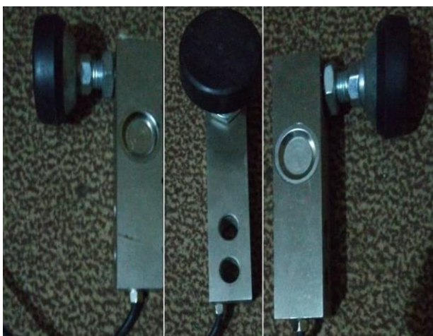
Fig. 8. Load cell (single-point 2,000 kg linearly defined load cell characterized by 0–20 kN of force with \pm 0.005\% accuracy).
