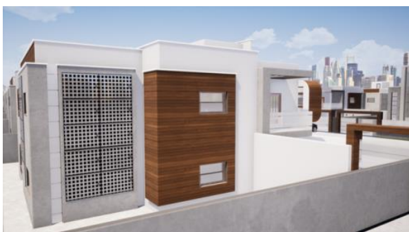
Fig. 39. The second integration of facades with PV modules (the researcher using sketch).
