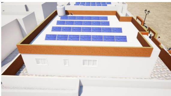
Fig. 22. Distributing the modules on the roof (developed by researcher).
