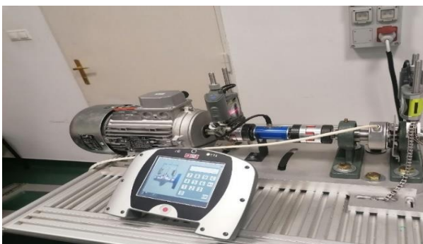
Fig. 3. Using Fixturlaser XA system to check the asynchronous motor alignment.
