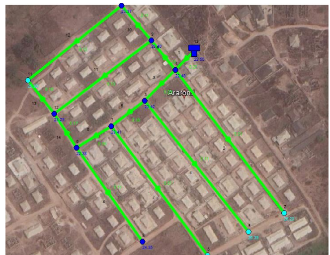
Fig. 2. Water Distribution Network for Araromi Community on EPANET 2.0 with backdrop from Google Earth.
