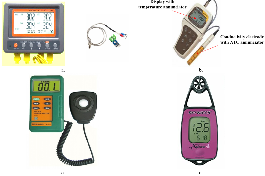
Fig. 4. Photograph of the instruments in the experiment setup; a) the data acquisition and k-type thermocouples, b) the conductivity / TDS device, c) the solar power meter, d) wind speed meter.
