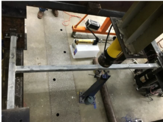
Fig. 2. Sub-assembly setup for quasi-static load test.
