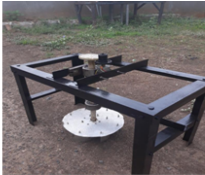
Fig. 13. Working prototype of the hydropower plant.
