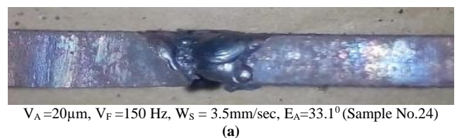
Fig. 16. Effect of electrode angle for different vibration frequency on bending strength
