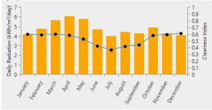
Fig. 2. The monthly average of solar radiation and clearness index
