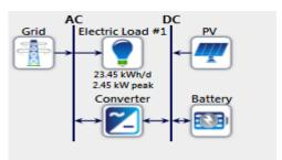
Fig. 5. Complete model of a grid connected PV power system
